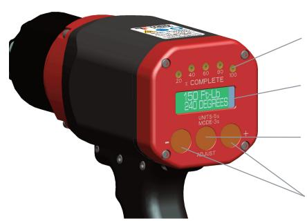
5 yellow LEDs indicate percent of set torque achieved. All LEDs turn green when set torque is reached and red if the set torque is not achieved.
