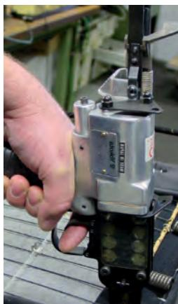
Pull the trigger and clamp. The work is completed when the trigger is released.
