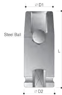
This wheel lug nut remover is used when it is discovered that the original key to remove your car wheel is lost. In order to remove the lock and the wheel, these sockets can be used. Proper use of the socket is to have at least three windings of thread of the socket gripping over the lock. In case any of the first three windings are already gripping, the next bigger size of socket should be chosen. When the correct size of socket is chosen, it can unlock up to four bolts.
